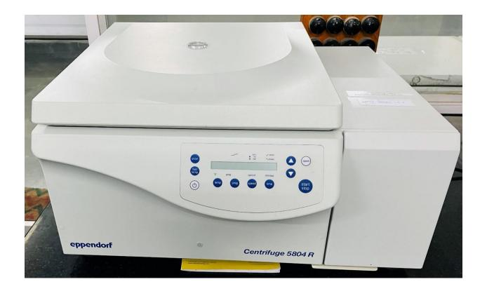
Instrument Name: Multipurpose Refrigerated Centrifuge
