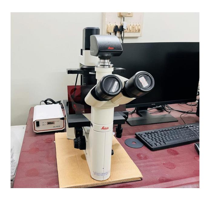
Instrument Name: Inverted Fluorescence microscope,
