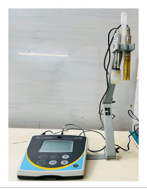
Instrument Name: Bench pH/mV/Conductivity/TDS/Temp. Multi-parameter Meter
